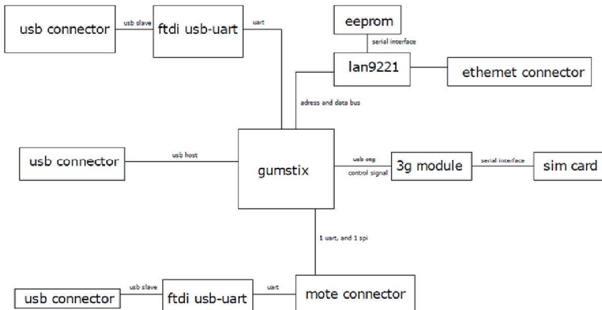
Figure 13 Main Component Block Diagram
