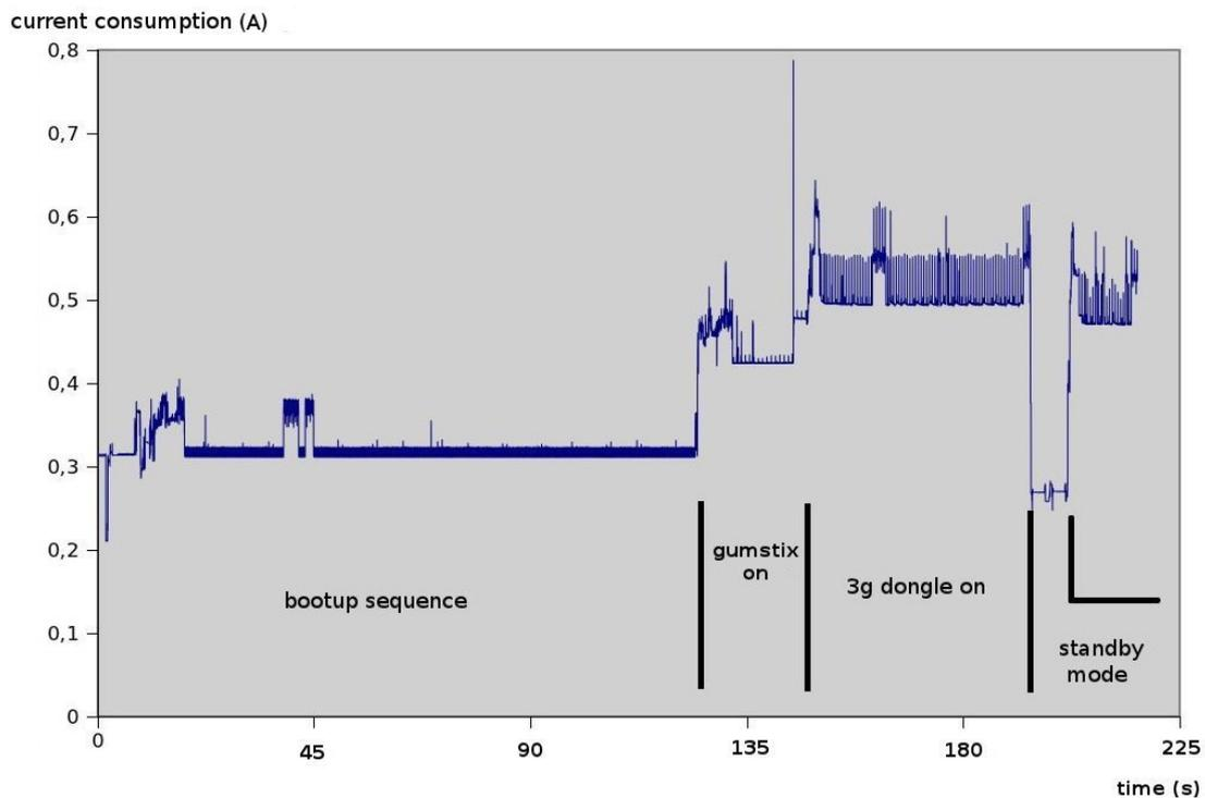
Figure 21: Preliminary Power Evaluation of the GENESI Gateway (various modes of operation)
