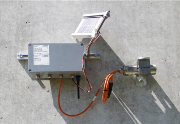
GENESI node with inclination sensor and solar panel
