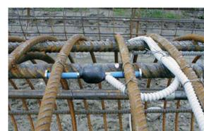
Figure 6: strain gauge
