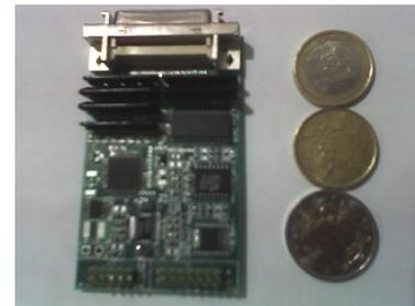
Figure 5: Interface with vibrating wire strain gauge
