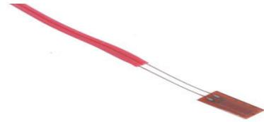
Figure 2: Resistive strain gauge
