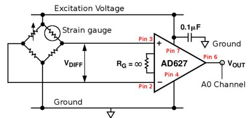
Figure 4: Interface to resistive strain gauge
