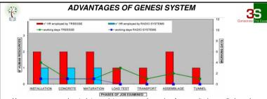
Human resources devoted to maintenance and repair of a monitoring radio-based system. We can see that the number of human resources devoted and the number of working days decrease substantially compared to a traditional cable-based monitoring system.
