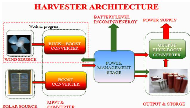
Figure 3 Solar harvester architecture
