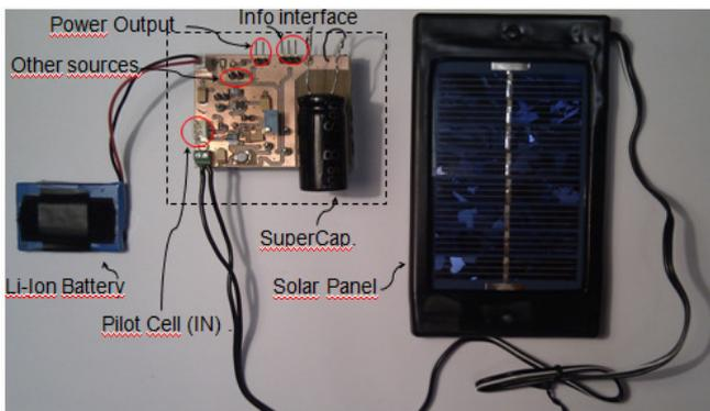
Figure 2 Solar harvester prototype
