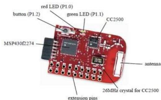
Figure 4 TI ez430-RF2500T test node.
